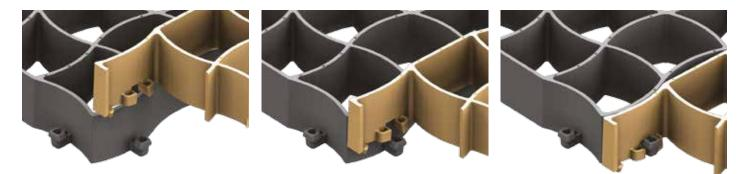
The innovative bayonet twist lock (male-female) simplifies installation and guarantees a perfect fixing of the grids. The characteristic "*Click*" iindicates that the connection has been successful. It is possible and recommended to preassemble the elements of the grid before positioning it, in order to speed up the installation.
