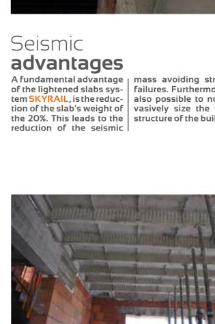
mass avoiding structural failures. Furthermore, it is also possible to non - invasively size the vertical structure of the building
